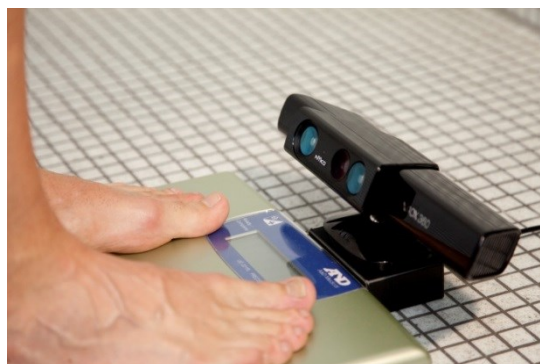
Figure 1 – Illustration of the sensor system, consisting of 3D camera and body weight scales (taken from [12])
