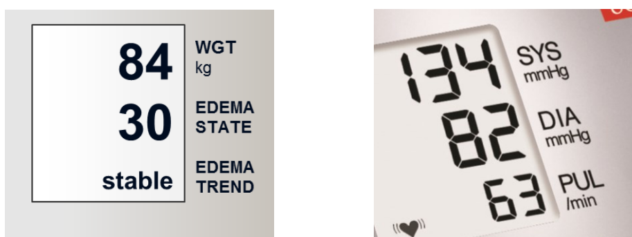
Figure 3. Display of an extended body weight scales with leg oedema score (left) as compared to the display of a state-of-the-art blood pressure measurement device (right).
